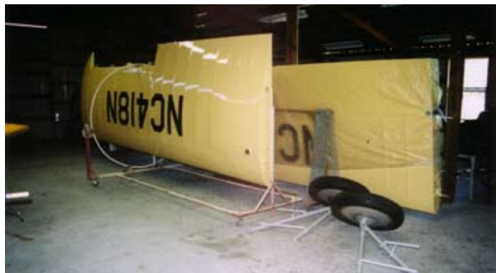
The 10-D wings are painted and ready to hang. These are large wings. Note the handling fixture. Photo by Jerry Impellezzeri.
