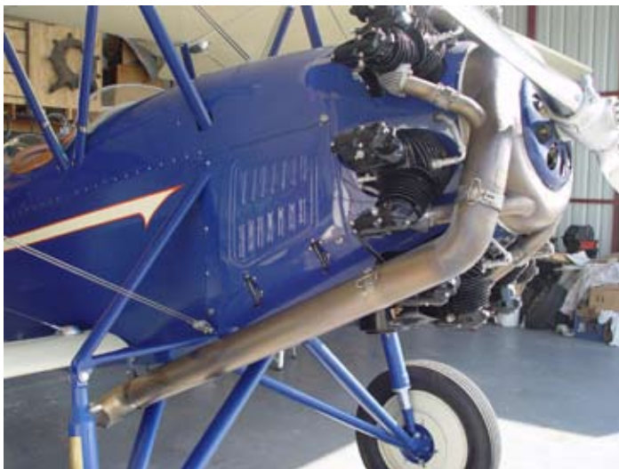
Bruce's 4D: Note the beautiful engine cowling work around the Wright J6-7
